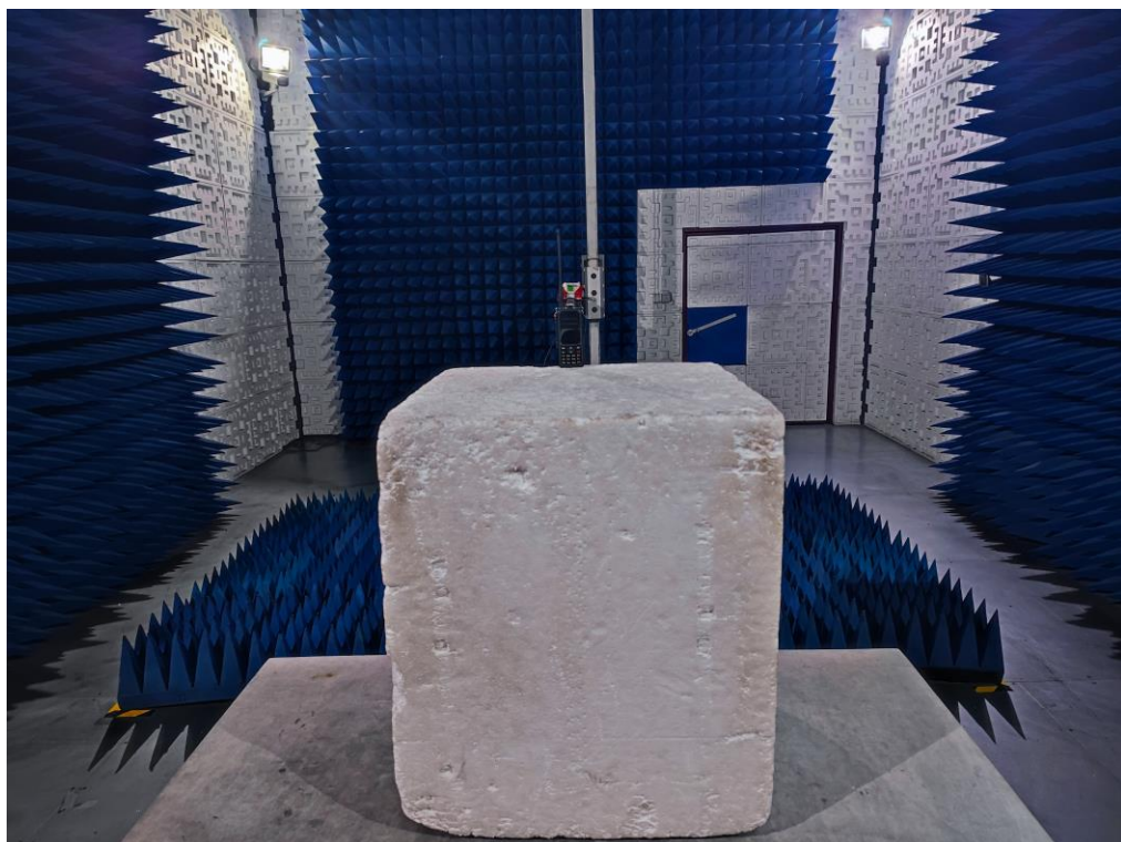
RADIATED SPURIOUS EMISSION ABOVE 1G TEST SETUP
