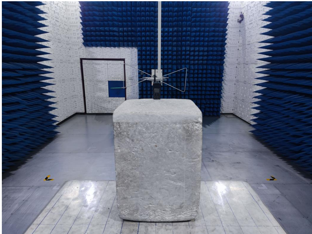
RADIATED SPURIOUS EMISSION ABOVE 1G TEST SETUP
